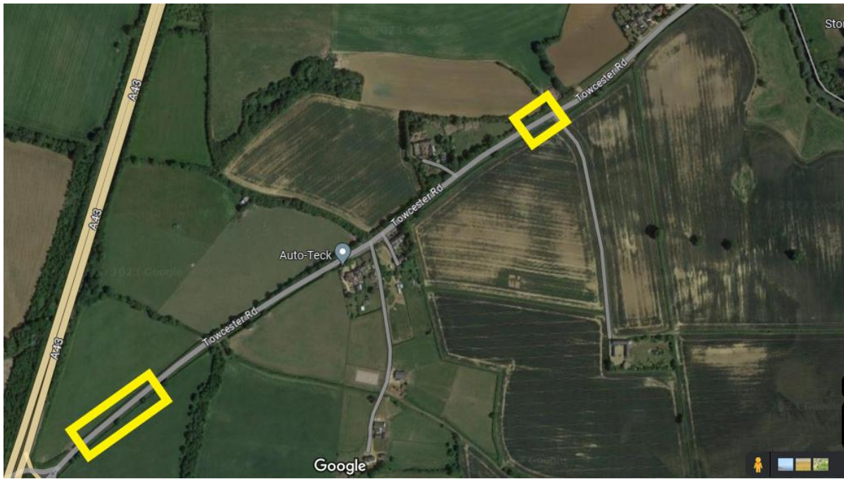
Proposed position rumble strips to slow the traffic down as they exit/join the A43.
